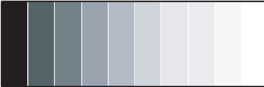
Figure 4-4. Typical Gray Bar Pattern for Adjusting Contrast
